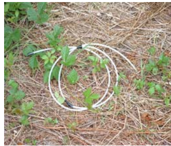
Above ground portion of piezometer. Photo courtesy of Jim Sutherland
